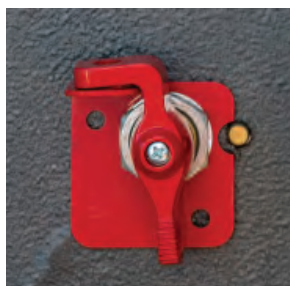
Isolation switch in OFF position
