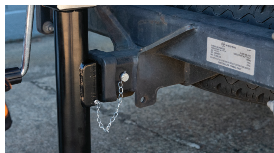
Figure-4 Secure the adapter with acceptable bolt/hardware
