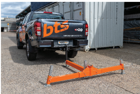
Level the base using the adjustable feet and spirit level on the base. The hitch mount davit base is now ready to use.
