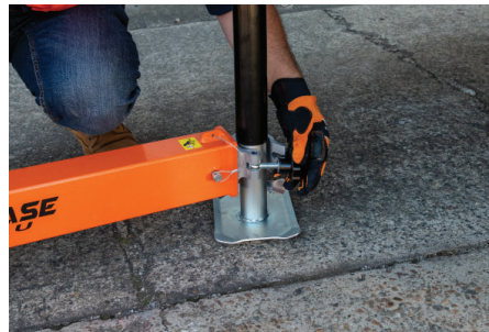
Rotate the crank handle on the jack foot to lift the rear of the vehicle to take weight off the rear wheels.
