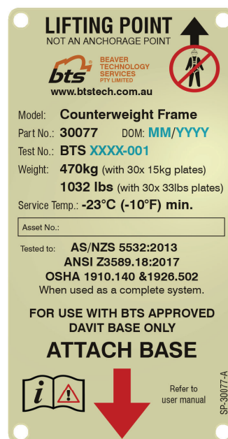
SP-30077-A Counterweight base ID Plate
