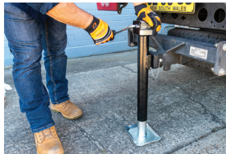
Rotate the crank handle on the jack foot to lift the rear of the vehicle to take weight off the rear wheels.
