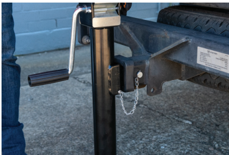
Rotate the crank handle on the jack foot to lift the rear of the vehicle to take weight off the rear wheels.
