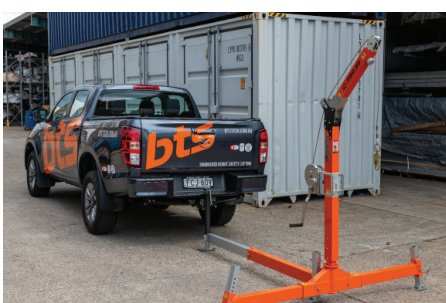
Level the base using the adjustable feet and spirit level on the base. The hitch mount davit base is now ready to use.
