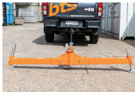
Level the base using the adjustable feet and spirit level on the base. The hitch mount davit base is now ready to use.
