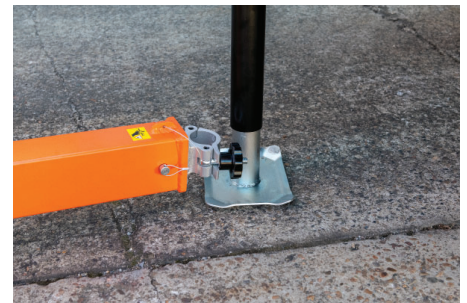
Position the hitch mount davit base at the rear of the vehicle with the coupler facing the installed jack foot.
