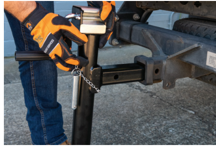
Remove tow hitch from vehicle and insert the jack foot into the hitch receptor.
