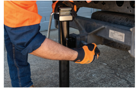
Insert the locking pin into the hitch receptor and jack foot.
