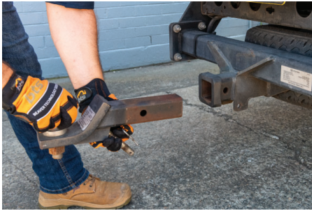
Remove tow hitch from vehicle and insert the jack foot into the hitch receptor.
