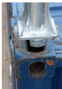
Place container post into ISO corner casting
